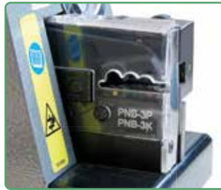
PNB-3P detail of the crimping zone.
