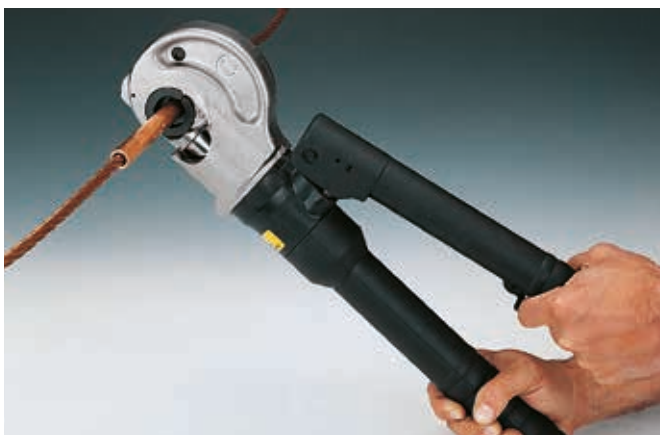
Die release system, protected from accidental operation
